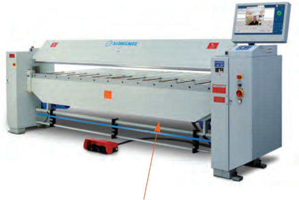
MAB and MAX – 16" folding beam width
